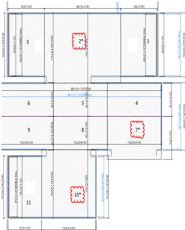
Figure 3. Floor Shop-Drawing Crop Showing Starred Oversize Pieces 2*, 7*, and 10* at Threshold and Drywall-Notch Conditions, where Added Material was Retained for Controlled Field Trimming at Recoverable Edges
